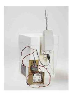
additional battery with a voltage range from 9 to 19 V. The recommended battery is a 9 V square battery that can easily be fitted onto the ozone sensor frame inside the ozone box.
